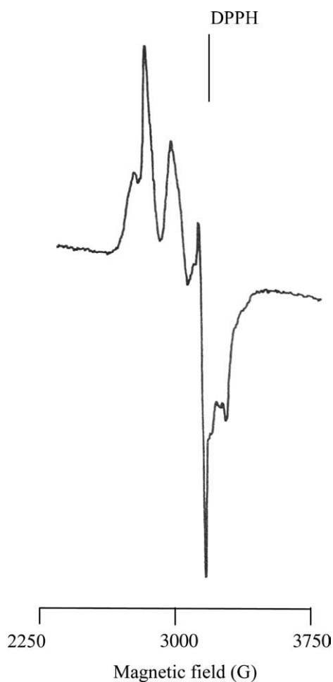
Fig. 3. EPR spectrum of the complex 7 in dichloromethane solution at 77 K.
